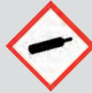
Gas under pressure
