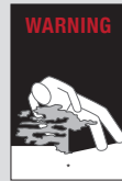
Carriers that contain agents for cooling or conditioning and which pose a risk of suffocation
